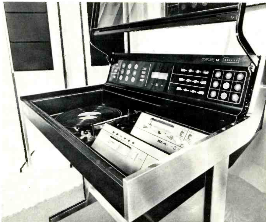
HOME AUDIO CENTER OF THE FUTURE , using speakers (seen left, beyond the console) that activate from across the room with signals from Infrared devices. It also uses touch-type electronic controls that light when contacted.
