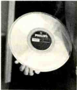
PHILIPS VIDEODISC is brightly silvered optical type used in their laser TV disc system.
